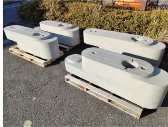
Photo 3. Precast concrete products (continuous foundation blocks for guardrail) manufactured by using CARBOCATCH slurry
