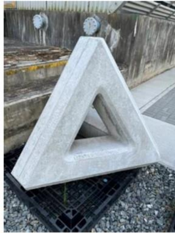
Photo 2. Wave-dissipating concrete block manufactured by using CARBOCATCH slurry
